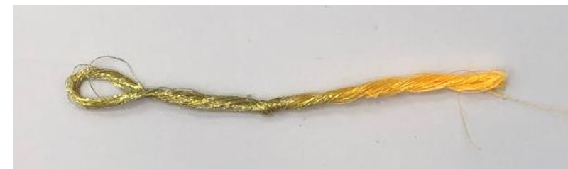
Regular metallic thread with silver plated metallic film, after dipping in household bleach for 5 minutes. The portion which is bleached has lost all the shine and color, only the core yarn is showing.
