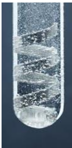
Aluminum reacting with alkaline solution
